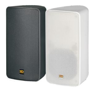
The RD 108T is a highly weather-resistant, single 8" 2-way full range loudspeaker, the body is made of engineering plastic injection molding. fitted with one 8" mid-woofer and one 1" HF driver. The system conforms to IP46 international standard. RD 108T is equipped with multi-tap transformer based on RD 108.
